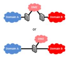
DMZs are used to prevent direct access to information and services on internal networks. DMZs usually provide a selection of information and services to less trusted networks, such as the internet. A DMZ does not necessarily provide additional security functionality, it simply provides a level of network separation for servers that must be made available externally. Therefore, a DMZ may be seen as both a type of security domain and type of trust zone.
