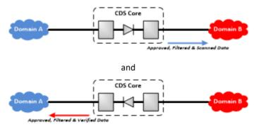
Note that the grey boxes in the above (and following) diagrams are intended to represent a generic collection of security-enforcing mechanisms within a CDS. The internal architectures of a real CDS may differ from this abstraction.
