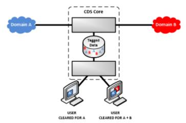
One key security feature of MLS systems is that users cannot directly access the connected security domains. Therefore, a MLS system could be desirable when users aren't cleared to the same level but need to work together with varying information within the same environment.
