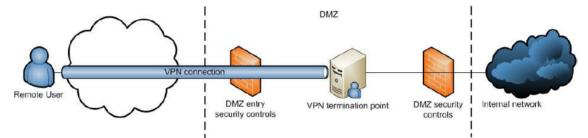
The following diagram shows a simplified example of an improper VPN connection termination within a DMZ.
