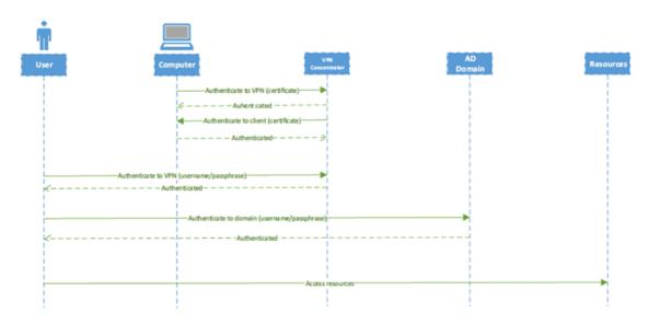
The risk associated with this scenario is that malicious actors may be able to compromise the computer's IPsec certificate at one point in time, compromise the passphrase the user uses to authenticate to the VPN concentrator at another point in time and, finally, compromise the user's AD credentials at yet another point in time. In this way malicious actors are able to increase their access over time, which increases the level of risk associated with this approach.
