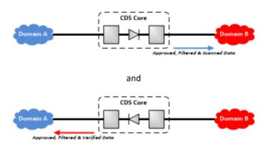
Note that the grey boxes in the above (and following) diagrams are intended to represent a generic collection of security-enforcing mechanisms within a CDS. The internal architectures of a real CDS may differ from this abstraction.
