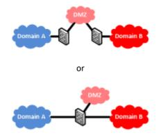
DMZs are used to prevent direct access to information and services on internal networks. DMZs usually provide a selection of information and services to less trusted networks, such as the internet. A DMZ does not necessarily provide additional security functionality, it simply provides a level of network separation for servers that must be made available externally. Therefore, a DMZ may be seen as both a type of security domain and type of trust zone.
