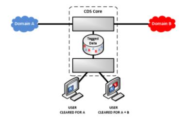
One key security feature of MLS systems is that users cannot directly access the connected security domains. Therefore, a MLS system could be desirable when users aren't cleared to the same level but need to work together with varying information within the same environment.
